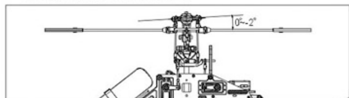
Stick position at low/Throttle 0%/Pitch 0°~2° 搖桿低速/油門0%/Pitch-2~0°
